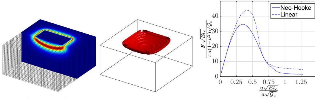
**Fig. 4:** Benchmark SPP1748, cf. [7], Final state, crack surface and force-displacement curve for the non-linear material model.
