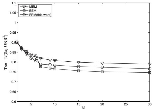
Fig. 3: Dimensionless shape factor  $T_s$  of torque for the rotation of a straight chain of  $N$  spheres around its major axis.
