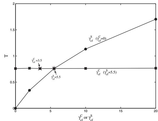
Fig. 1: Dependence of torque on the sphere exerted by the fluid on the value of: 1)  $\gamma_{cf}^S$  when  $\gamma_{cf}^C = 0$ , and: 2)  $\gamma_{cf}^C$  when  $\gamma_{cf}^S = 5.5$ . Here  $\Omega = -0.4$ .
