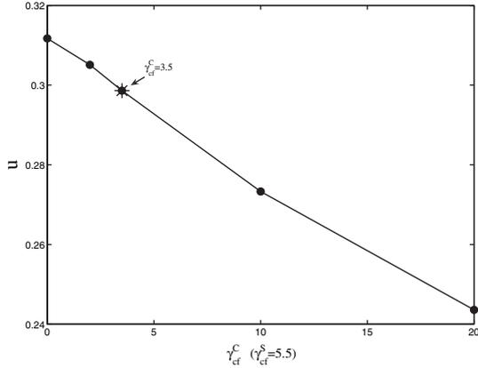
Fig. 2: Dependence of the superficial velocity of the fluid on the value of  $\gamma_{cf}^C$  when  $\gamma_{cf}^S = 5.5$  in the unbounded uniform Stokes flow around one sphere.
